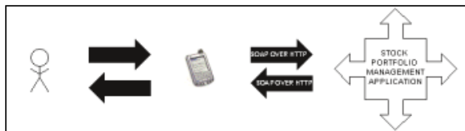
FIGURE 2 Using a SOAP client application on a PDA to interact with a Stock Portfolio Management Application
